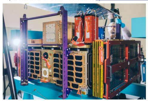
Photograph of the Vigoride orbital transfer vehicle with customer payloads at Momentus headquarters before being shipped to Cape Canaveral for integration with the SpaceX Falcon 9 launch vehicle. Photo Credit: Niall David
