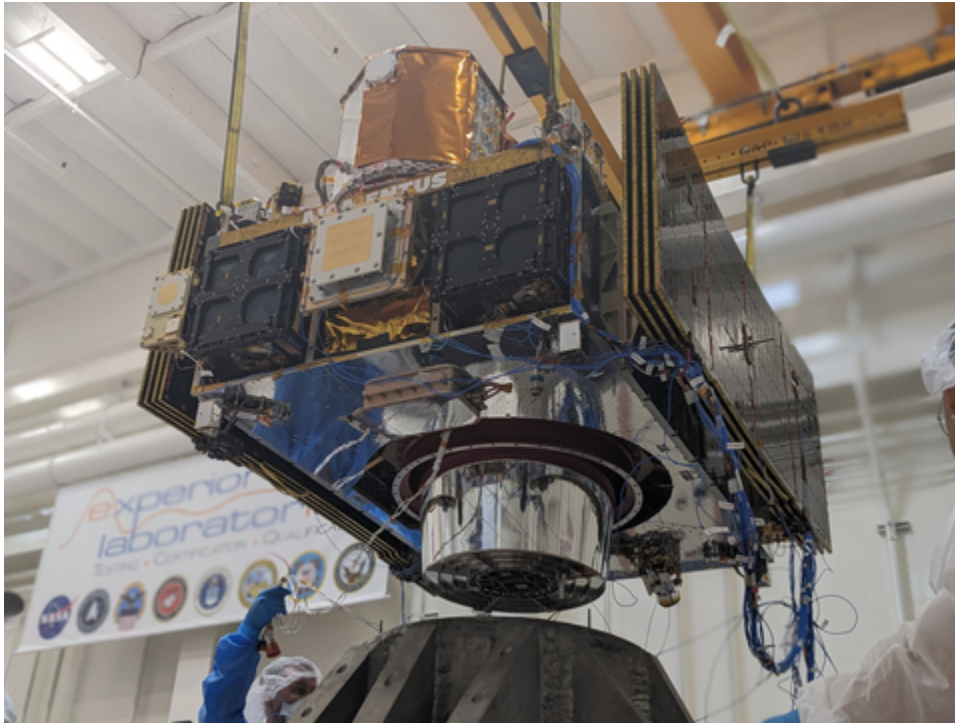
Momentum's Vigoride-7 Orbital Service Vehicle undergoing vibration testing at Experior Laboratories. (Photo: Momentum)
