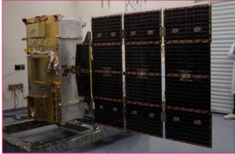
Solar Array Deployment Testing
