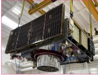
Thermal Vacuum Testing
